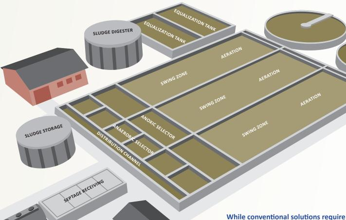
diffusers, blowers, motive pumps, impellers, and more, BioMix utilizes a centralized compressor system that minimizes maintenance and maximizes energy efficiency.
