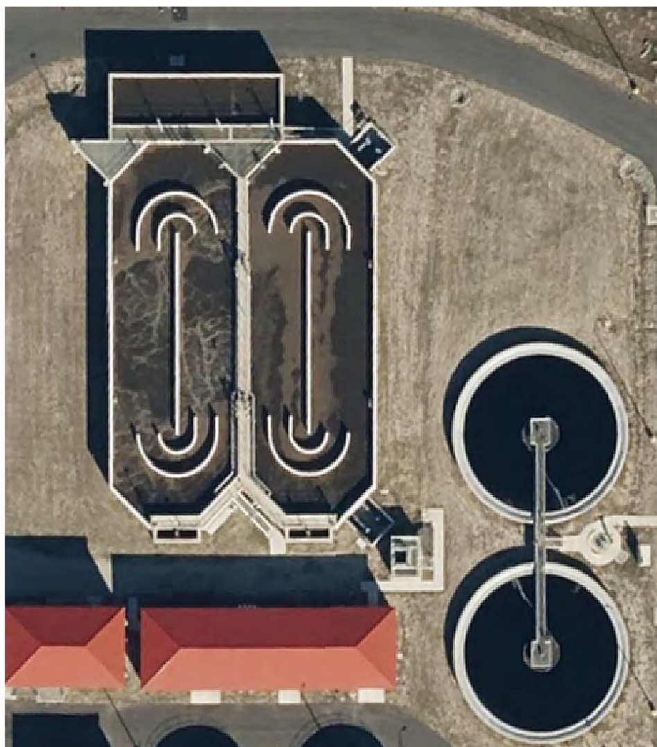
Dual Continuous Loop Reactors with Clarifiers
